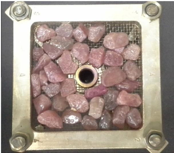
Fig. 7. Natural sapphire stones are held in the sample holder for ion implantation.
