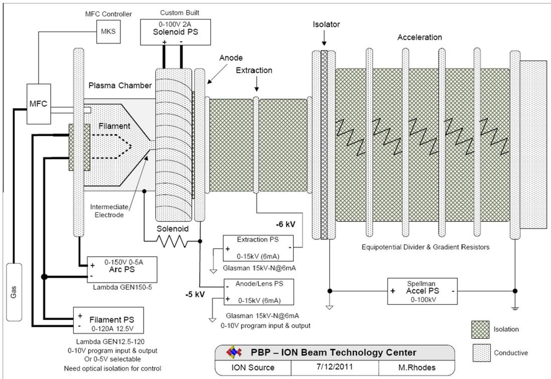
Fig. 2. Schematic diagram of high-voltage terminal system including the duoplasmatron ion source and the home-modified accelerating tube with their power supplies.
