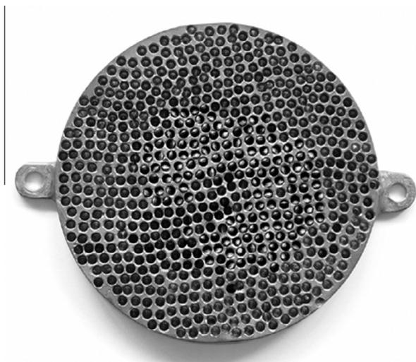
**Fig. 5.** Photograph of the specially designed rice seed sample holder. Rice seeds are being held in the holes of the holder.
